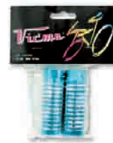
Ref. 586 Reposapias BMX-Free Style. Aluminio. Ø26 mm. Longitud 75 mm. Rosca 24T x 26T (5/16" - 3/8").
